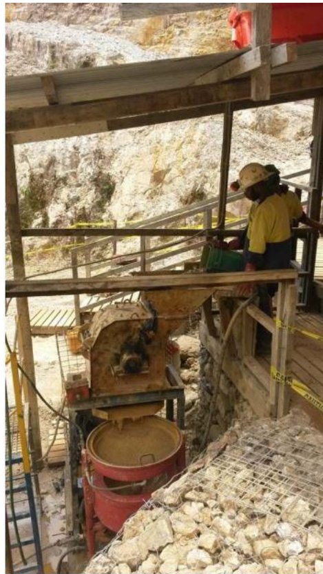
Figure 45: Hammer Mill and Centrifugal Gravity Concentrator. (Source: ASX: CGN 30 June 2015 Quarterly Activity Report)
