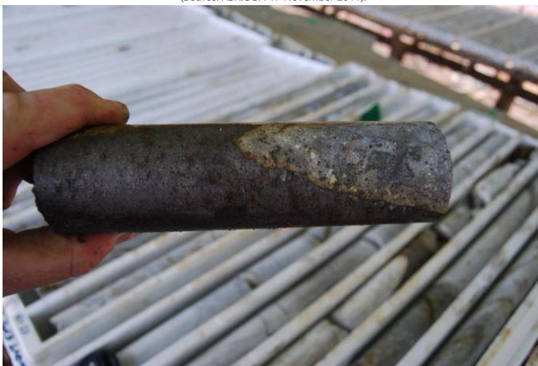
Figure 32: NEV027 drill core at 1046m depth: Massive pyrrhotite veining at the contact between the overlying Chim Formation and the felsic tonalite intrusive.
