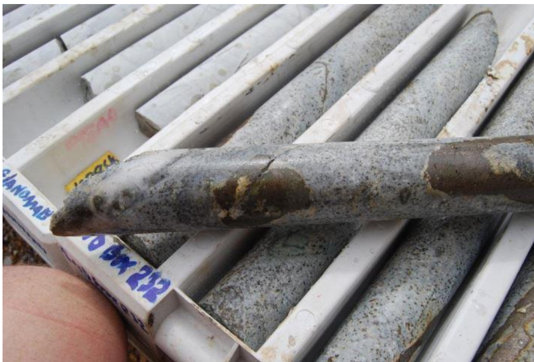
Figure 31: NEV027 drill core at 1076m depth. Felsic tonalite intrusive with quartz - base metal veining and fine disseminated chalcopyrite in groundmass.
