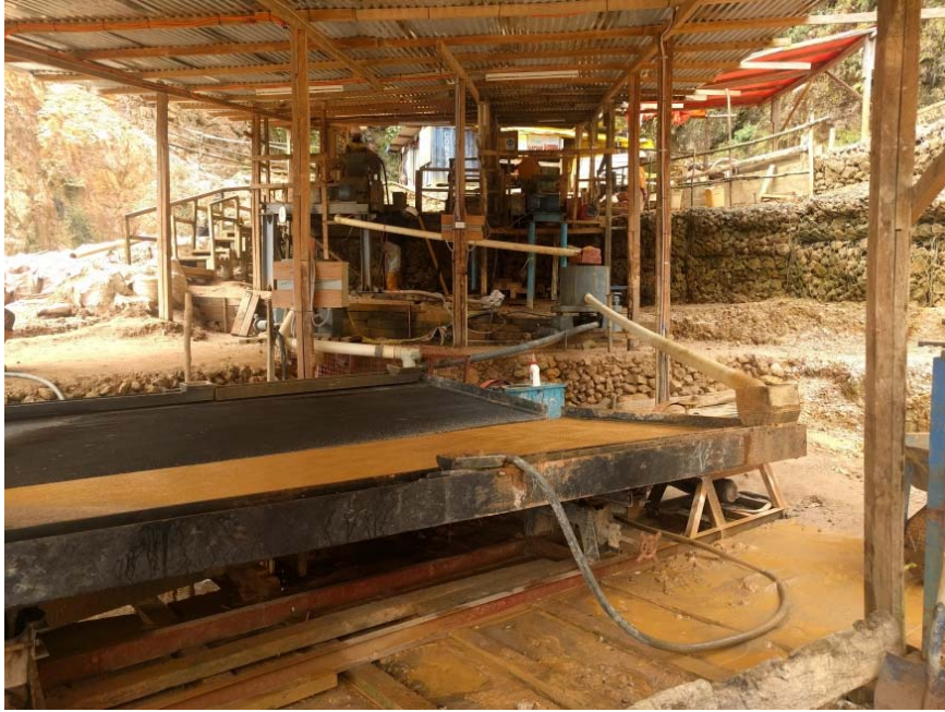
Figure 2 - Hammer mills, centrifugal concentrators and shaking tables
