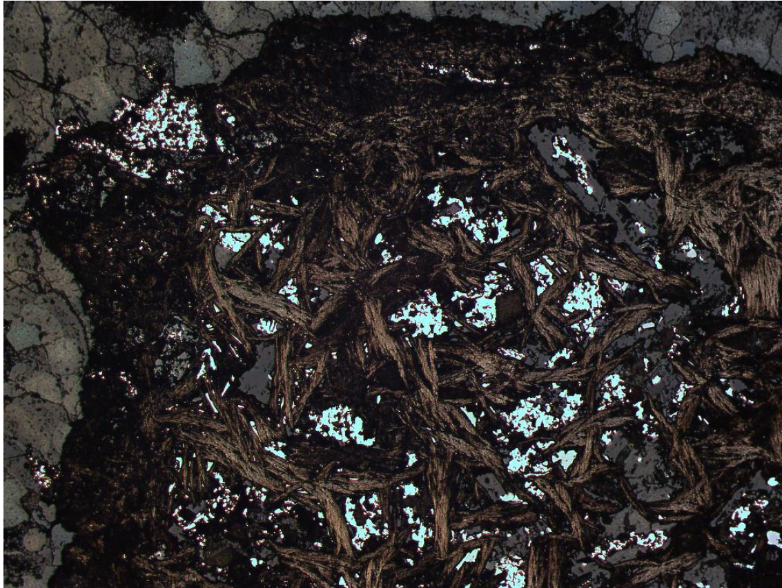
Polished Section 2: Reflected light [25x Mag. F.O.V. 4.8 mm] Coarse graphite flake - (Brown in colour)
