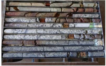
Figure 8- Graphite mineralisation from approximately 29.3m from the 1st drill hole
