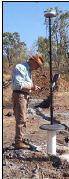
Figure 1.1 Hemisphere GPS Equipment In Use Surveying Drill Collars
