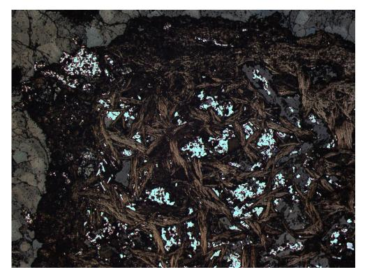
Figure 2: Polished Section 2: Reflected light [25x Mag., Field of view 4.8 mm] Coarse graphite flake - (Brown in colour)
