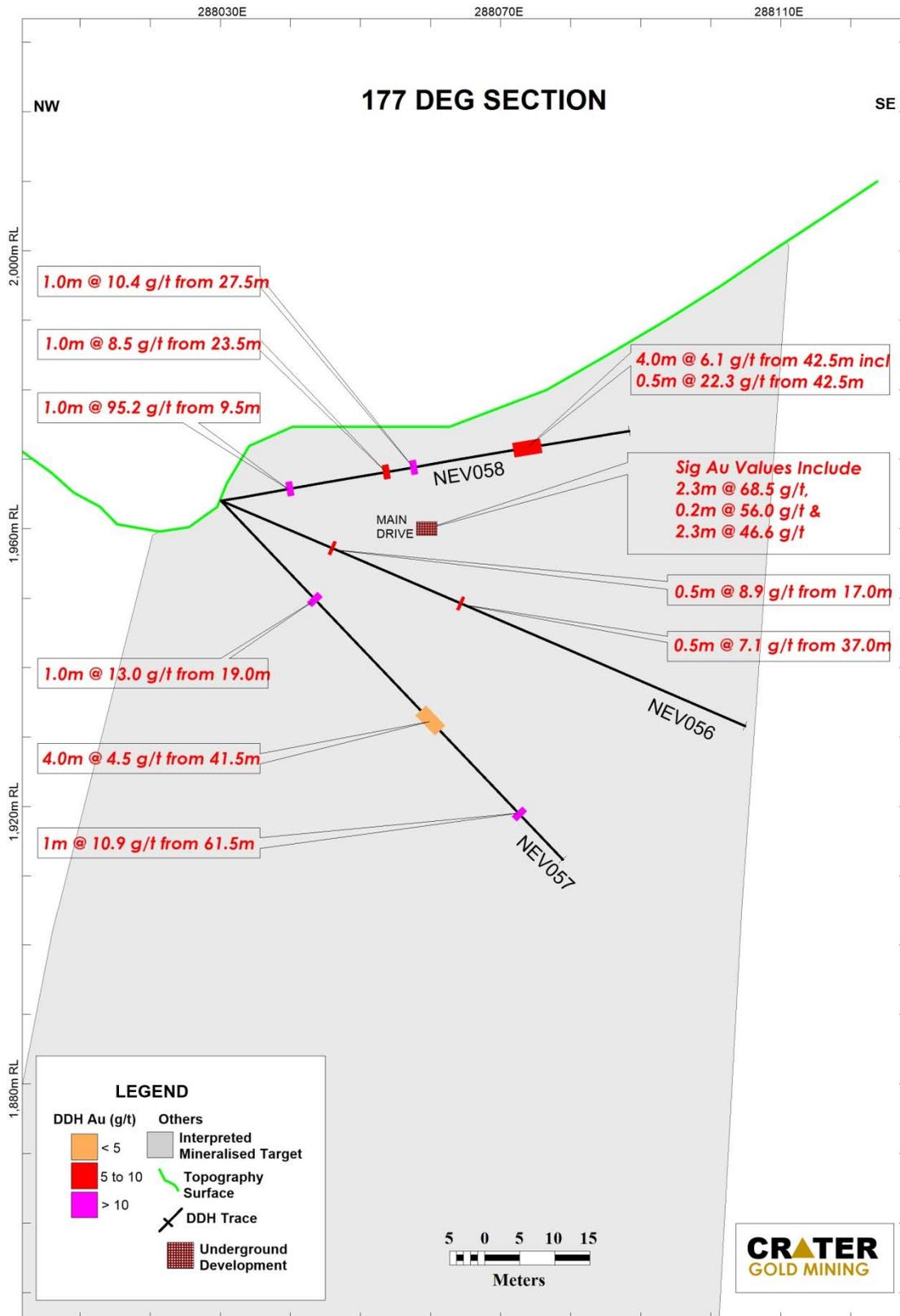
Figure 4 - Section of Drill Holes and Intercepts on 177° Bearing
