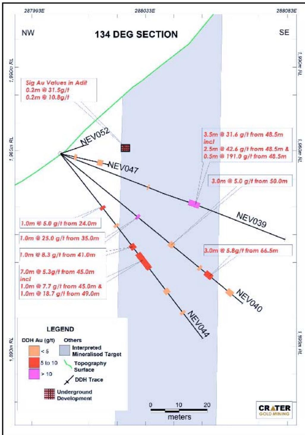
Figure 9 - Section of Drill Holes and Intercepts on 134° Bearing
