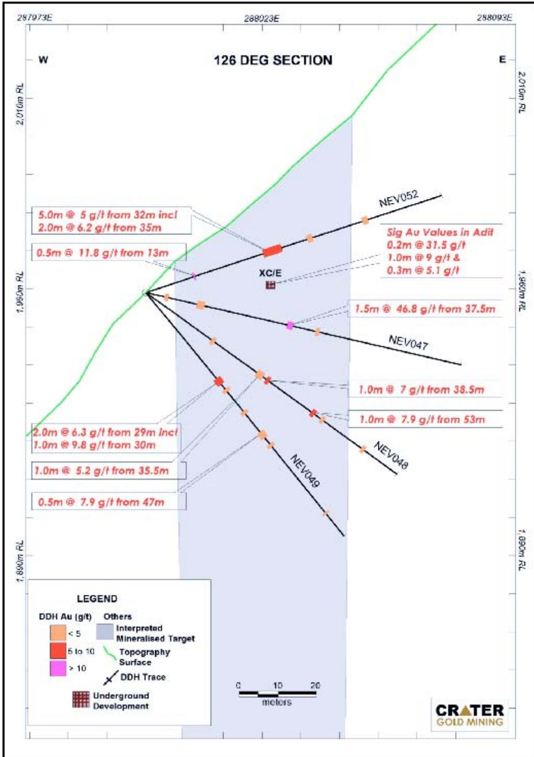
Figure 8 - Section of Drill Holes and Intercepts on 126° Bearing
