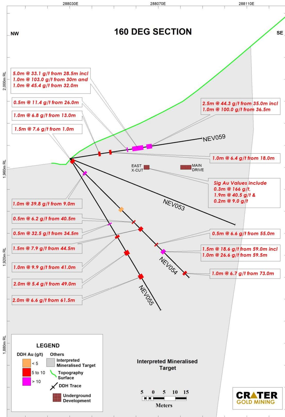
Figure 3. - Section of Drill Holes and Intercepts on 160° Bearing
