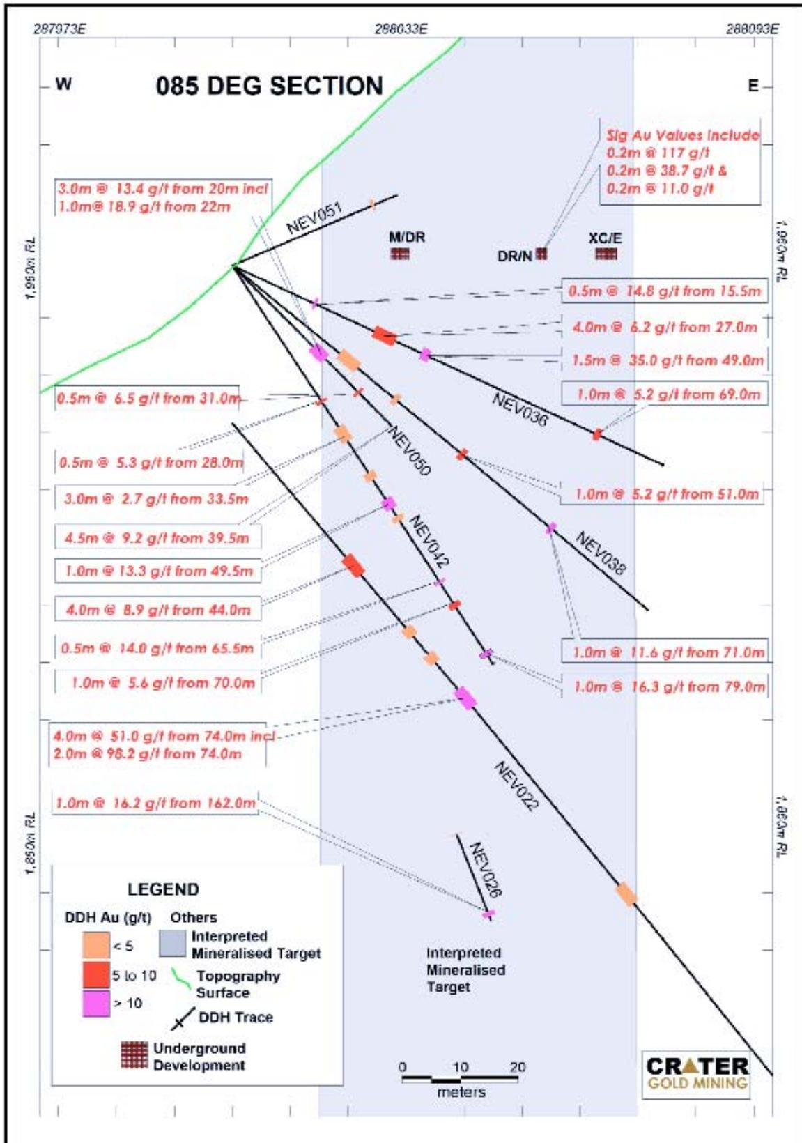
Figure 5 - Section of Drill Holes and Intercepts on 85° Bearing
