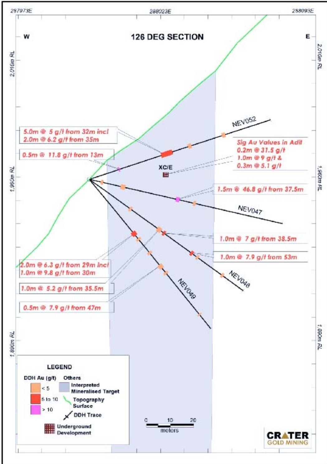
Figure 10 - Section of Drill Holes and Intercepts on 126° Bearing
