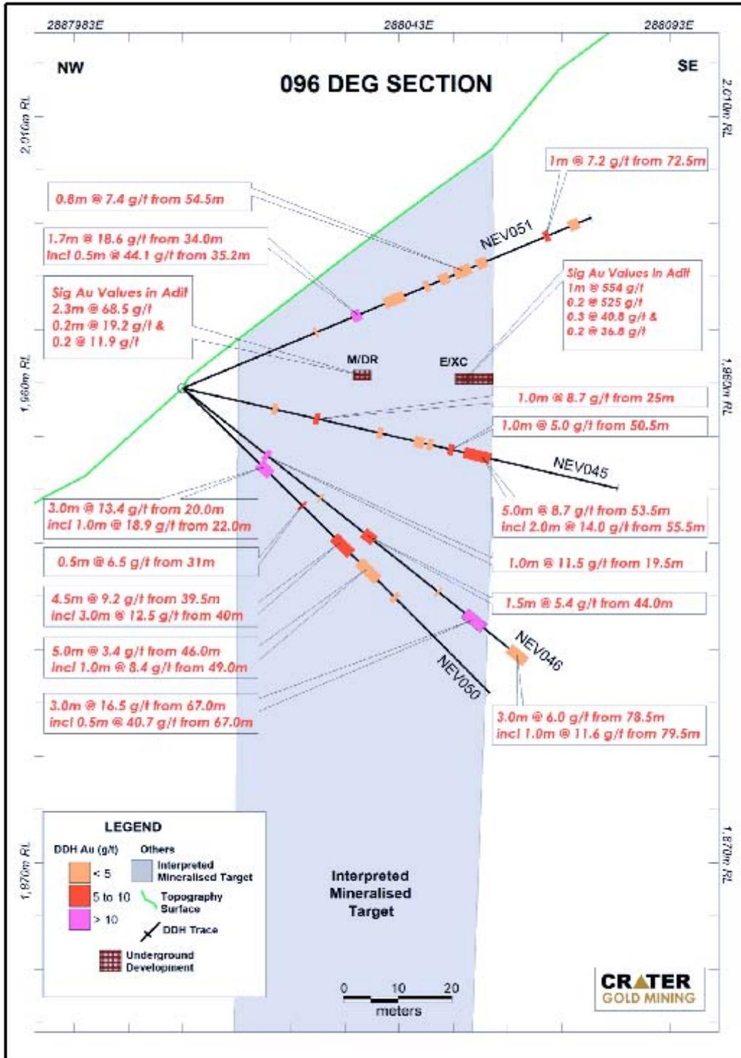
Figure 8 - Section of Drill Holes and Intercepts on 96° Bearing
