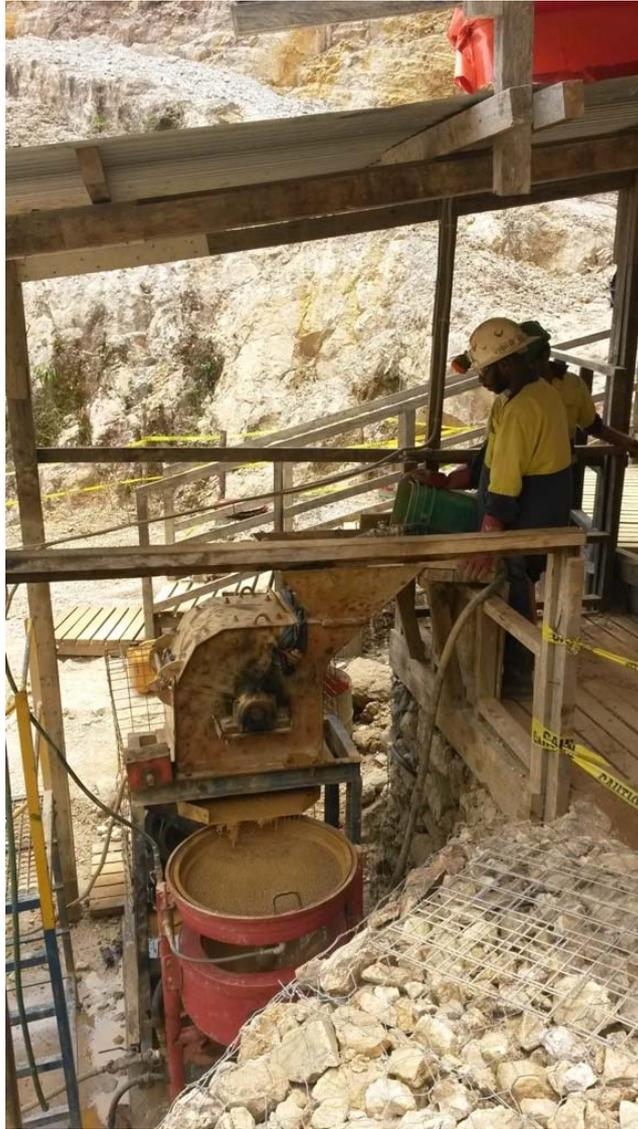
**Figure 1 - Hammer Mill & Centrifugal Gravity Concentrator**
