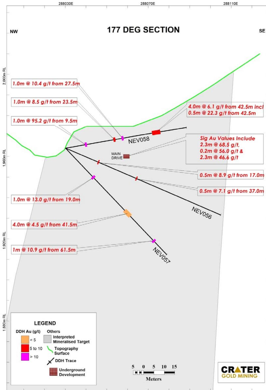
Figure 6 - Section of Drill Holes and Intercepts on 177° Bearing
