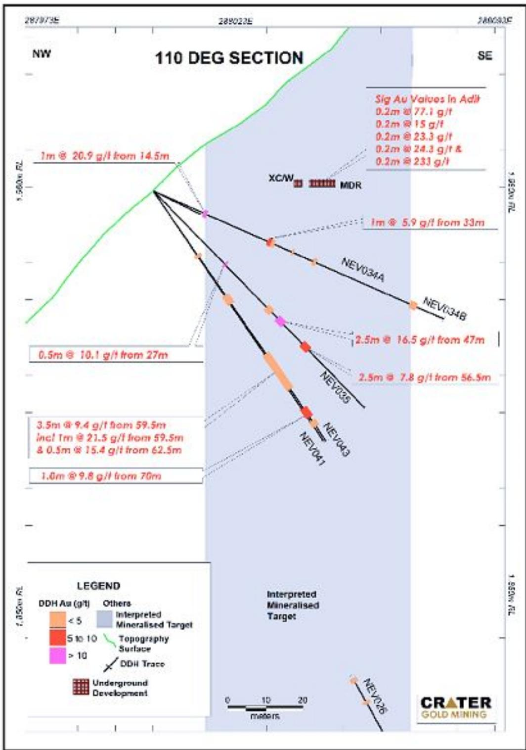
Figure 9 - Section of Drill Holes and Intercepts on 110° Bearing
