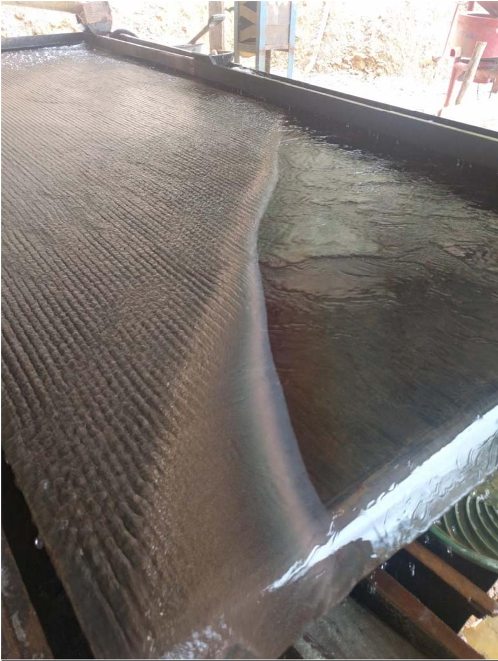
Figure 3 - Shaking table concentrate stream
