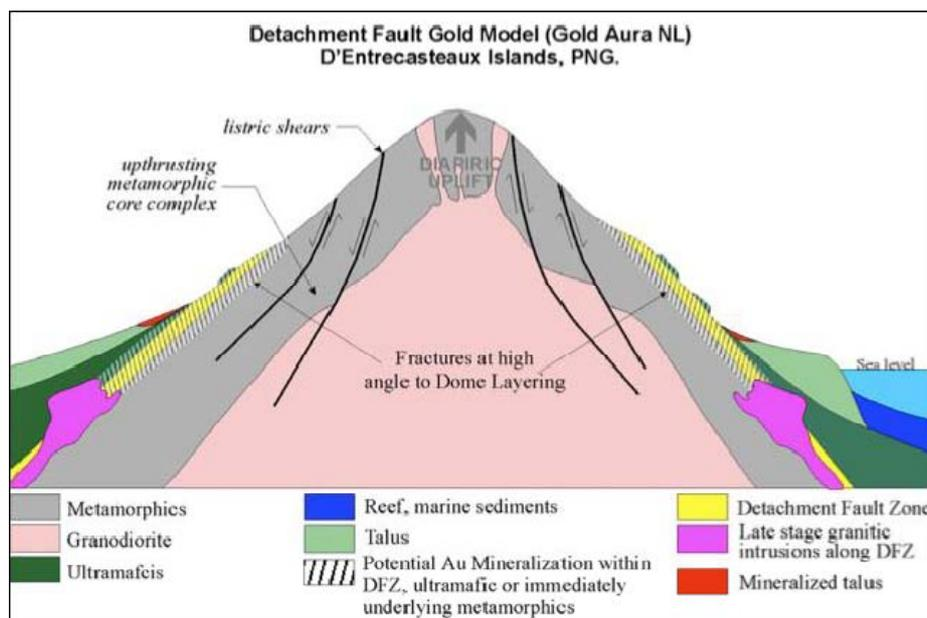
Figure 2 –Mineralisation model
