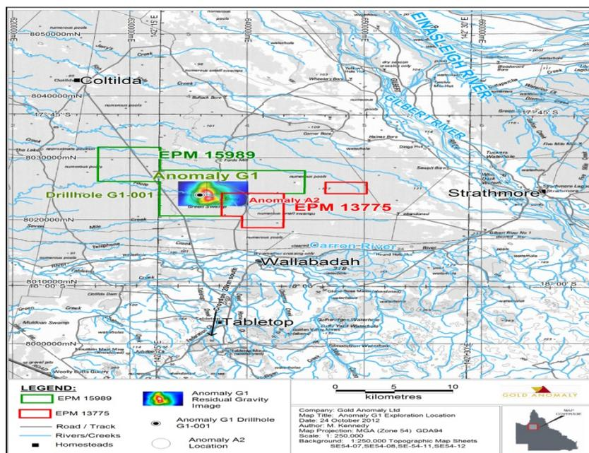
**Figure 6-** Location Map of the G1 Anomaly showing Residual Gravity and location of the G1 drill hole completed with the assistance of the CDI grant.
