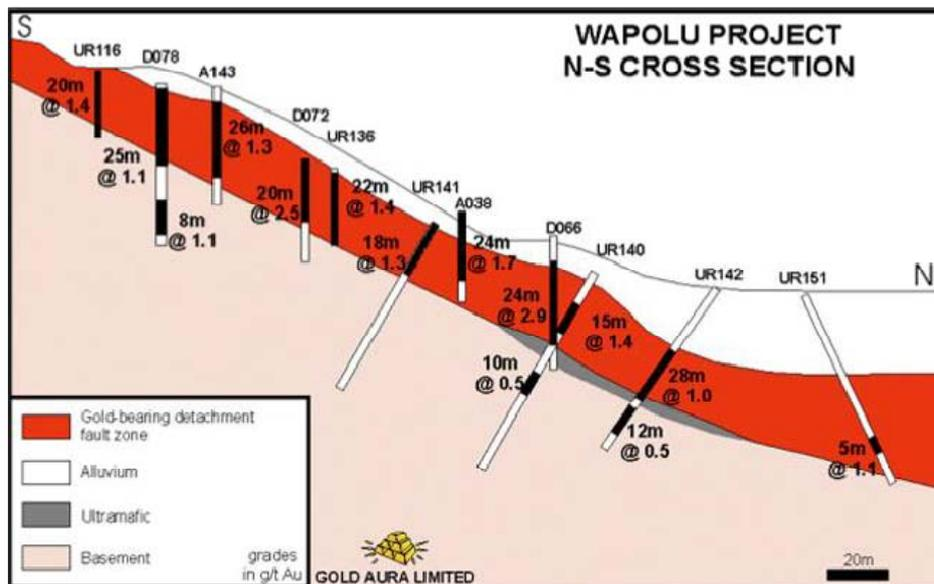
Figure 4 –N-S Drilling cross-section
