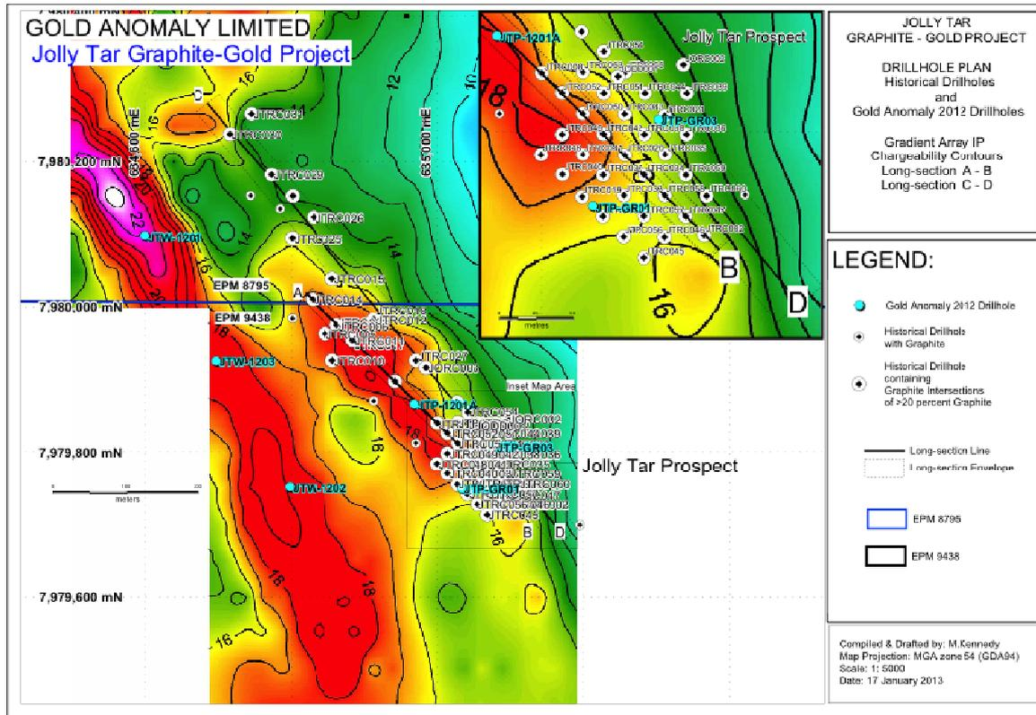
**Figure 5-** Drill hole plan showing graphite intercepts and gradient array IP anomalies at the Jolly Tar Prospect.
