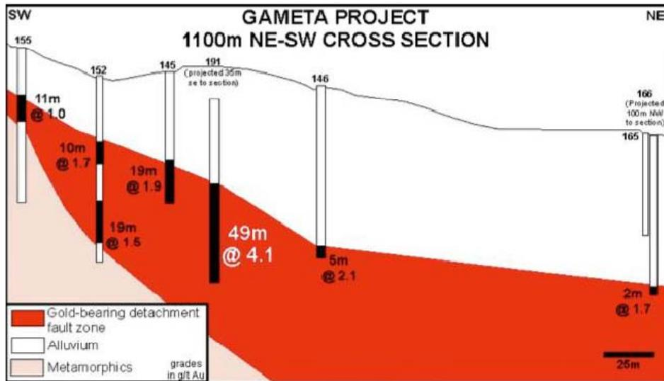
Figure 3– NE-SW Drilling cross-section
