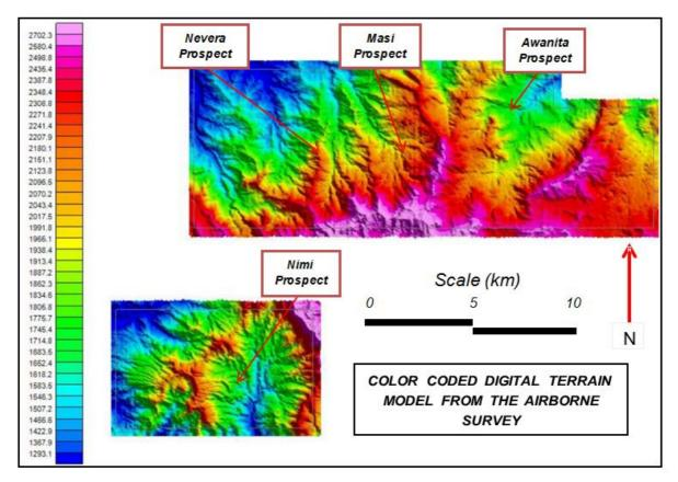
Figure 9 - Digital Terrain Model of the surveyed area (elevations are colour coded from blue - below 4,200feet/1,290m asl - to pink - above 9,000 feet/2,740m asl)
