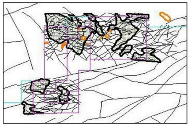
Figure 10 - Magnetic Interpretation Plan showing magnetic lineaments (black), areas of magnetite destruction or non-magnetic cover (green) and possible stock-like bodies (orange)
