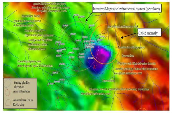
Figure 2 - TMI/RTP image displays CM-2 as negative magnetic field anomaly E of mineralised intrusive/magmatic hydrothermal system
