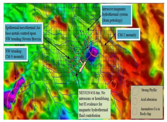
Figure 6 - TMI/RTP image showing projected SW plunge and NW dip of causative intrusion and related intrusive breccia
