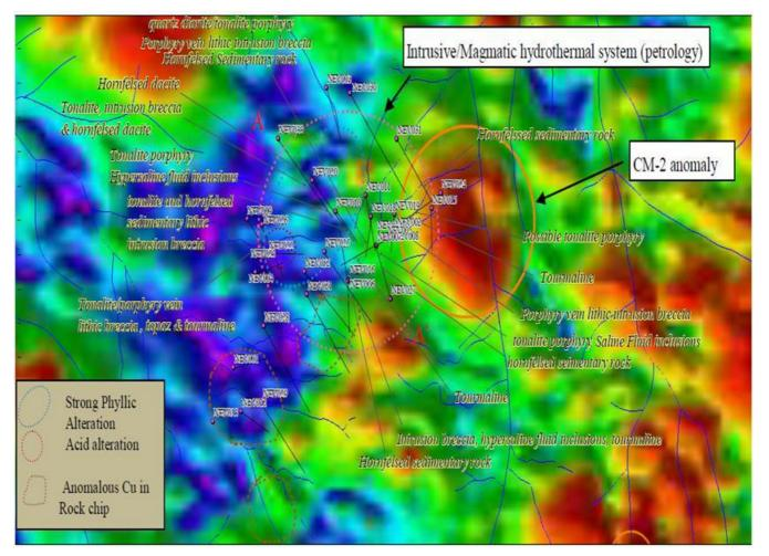
Figure 3 - TMI/AS image displays CM-2 as positive magnetic field anomaly E of mineralised intrusive/magmatic hydrothermal system
