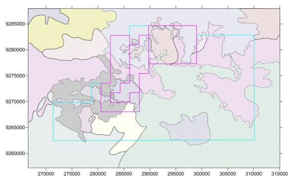
Figure 13 - Soil and exposed rock type interpretation from radiometric data Note: Colour code based on the dominant radioelement present using the same colour distribution as the Ternary Image.
