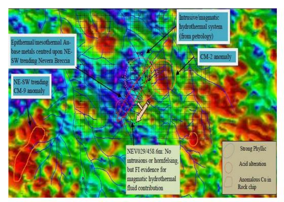
Figure 7 - TMI/AS image showing projected SW plunge and NW dip of causative intrusion and related intrusive breccia
