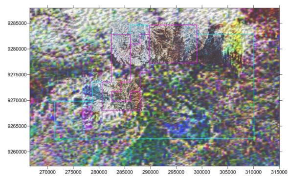
Figure 12- Ternary Radiometric Image (potassium - red, uranium - blue, thorium - green) Note: Strong contrasts are obvious between different geological areas as are differences between the Crater Gold (fine detail) and Fugro (coarse detail) surveys
