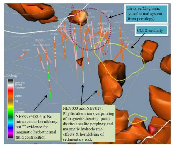
Figure 4 - 3D inversion model shows CM-2 with petrologically defined intrusive/magmatic hydrothermal system (oblique view from the SE)
