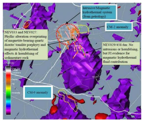
Figure 5 - 3D inversion model defining possible NE-SW trending magnetite bearing intrusive rocks (oblique view from the SW)
