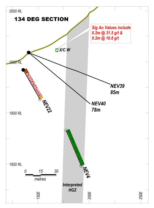
Figure 4. Section of Drill Holes and Intercepts on 134° Bearing
