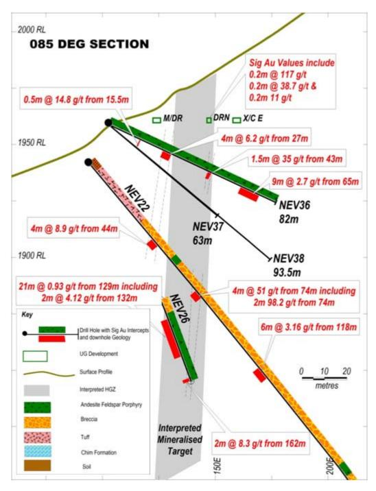
Figure 3. Section of Drill Holes and Intercepts on 85° Bearing
