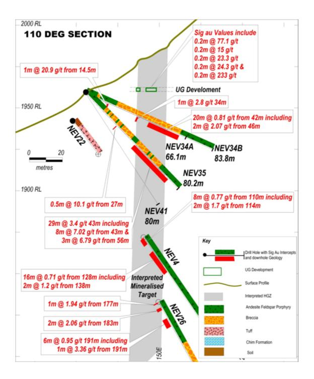
Figure 2. Section of Drill Holes and Intercepts on 110° Bearing
